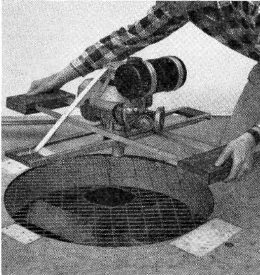
**MOTOR MOUNT** is bolted through the deck and upper main frame. Hardwood blocks clamping ends of each pair of angles add rigidity to the mounting assembly.
