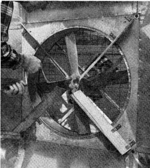
**PROPELLER MUST BE BOLTED** to the hub after the engine is in place. Vanes were added after the first trials to counteract torque effect and improve the air flow.
