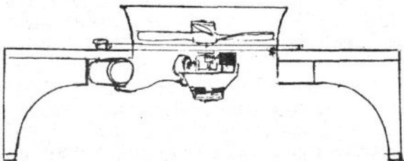
**INVERTING THE ENGINE** would lower center of gravity and allow use of standard prop with an engine rotating in conventional direction.
