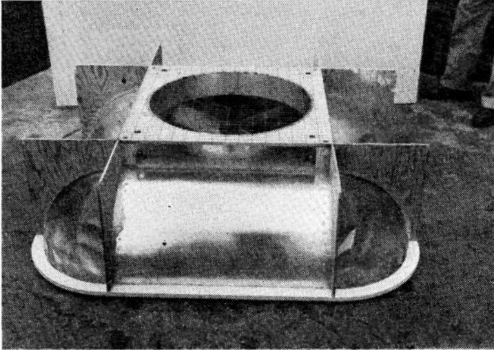
**FINISHED "HULL"** showing how fan shroud and rounded contours in the plenum chamber are obtained, using sawed-to-shape plywood covered with a skin of sheet aluminum and plastic film.
